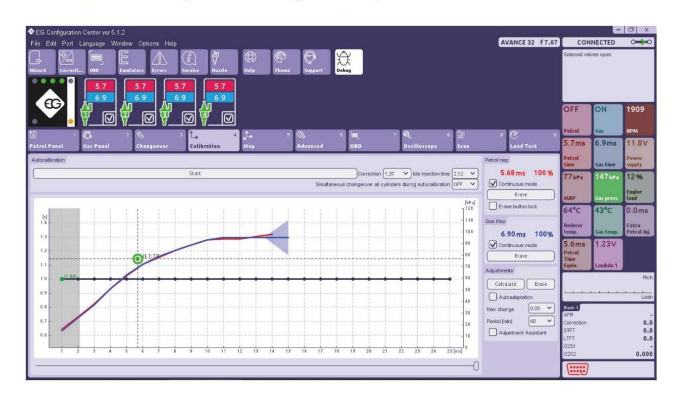
■ 1 Go for a test drive to collect gas map (blue colour) in full range of loads (drive until 100% of map will be collected).
