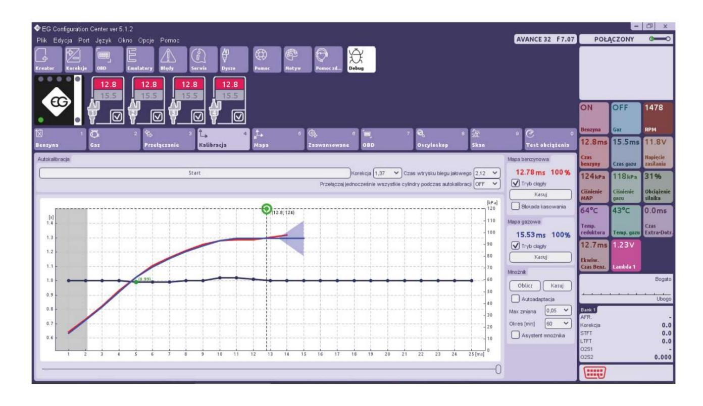
If petrol and gas maps are not close enough to each other, press Calculate adjustments button to adjust multiplier line.
