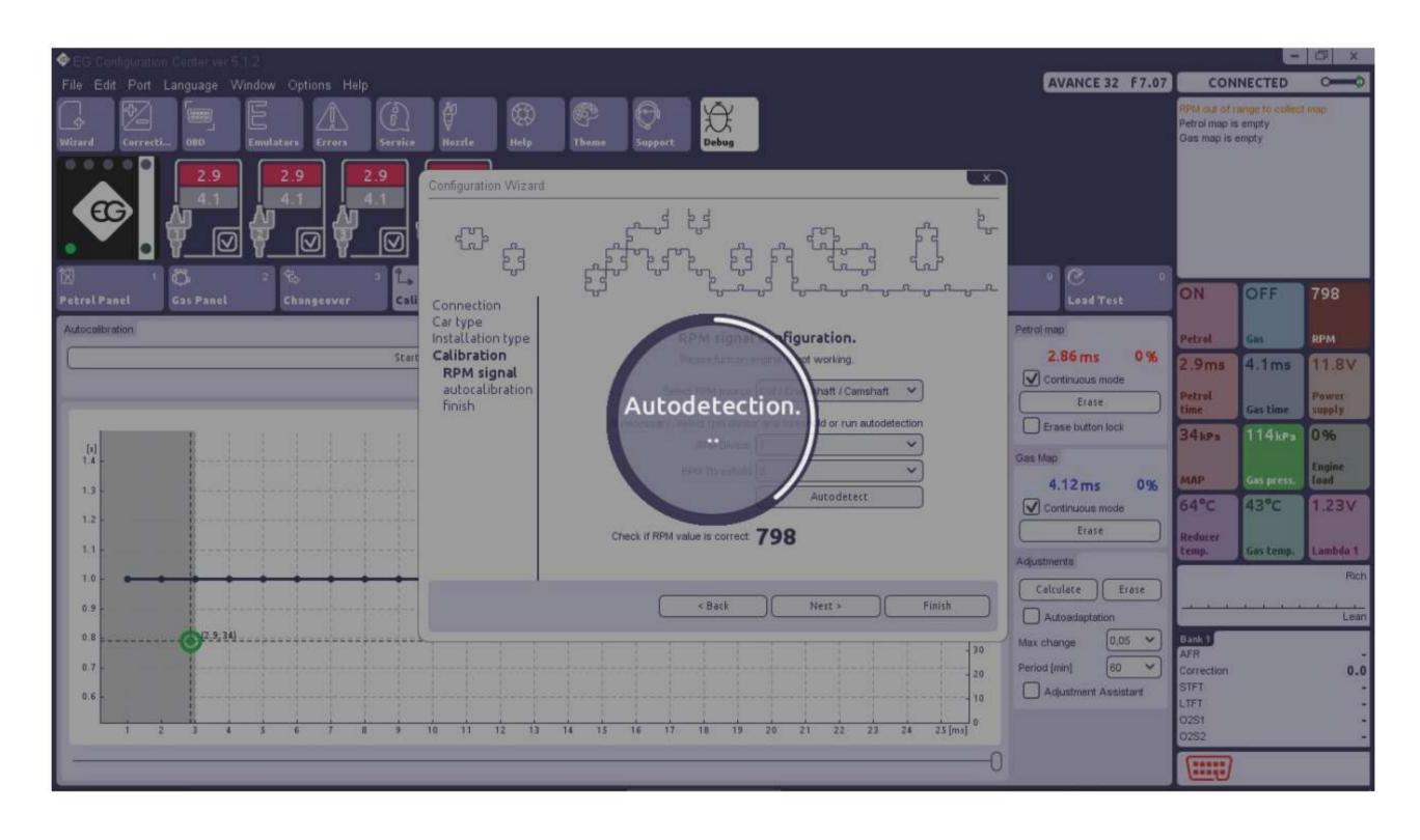
1 Press Autodetectbutton in order to allow ECU to detect correct RPM signal divisor and threshold automatically.
