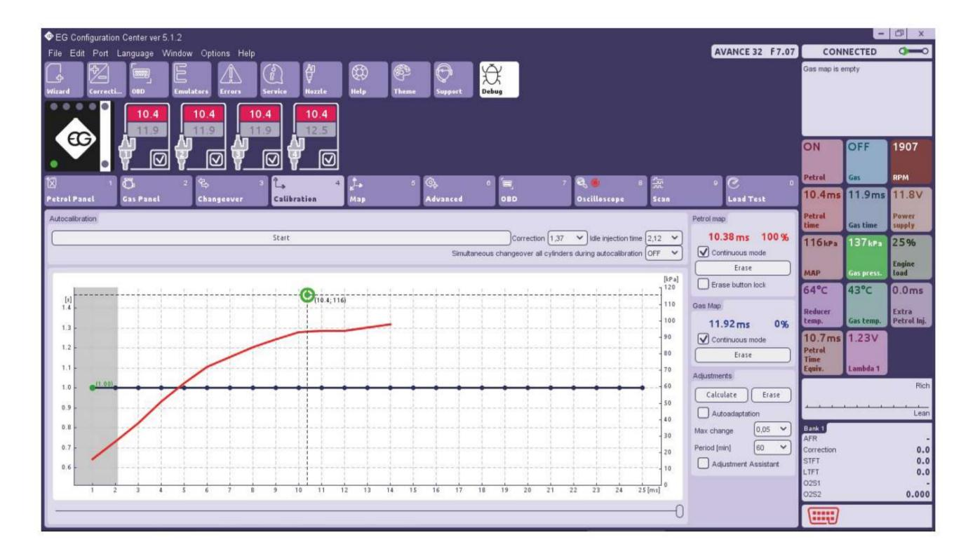
1 Go for a test drive to collect petrol map (red colour) in full range of loads (drive until 100% of map will be collected).
