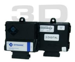
**EG DYNAMIC** Timing advance processor dynamically changes the moment of engine's ignition while it is running on LPG/CNG fuel to improve combustion process efficiency. This way vehicle's engine works more dynamically. Power losses during acceleration are practically eliminated.
