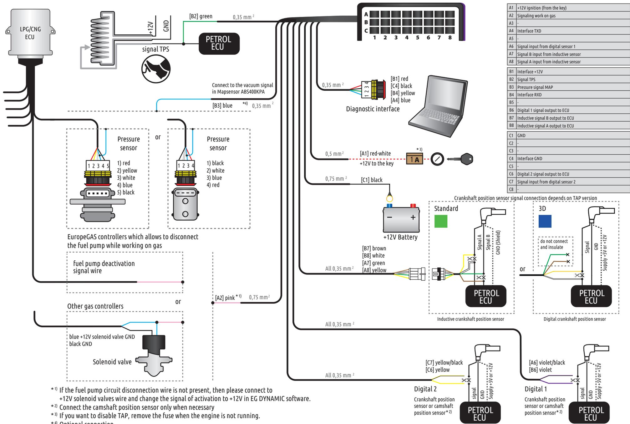
\*1) If the fuel pump circuit disconnection wire is not present, then please connect to +12V solenoid valves wire and change the signal of activation to +12V in EG DYNAMIC software.
